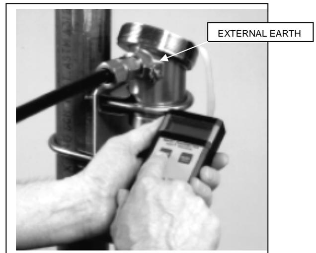
Once the first unit is configured, simply unplug the D-CAL unit and move onto the next unit.
